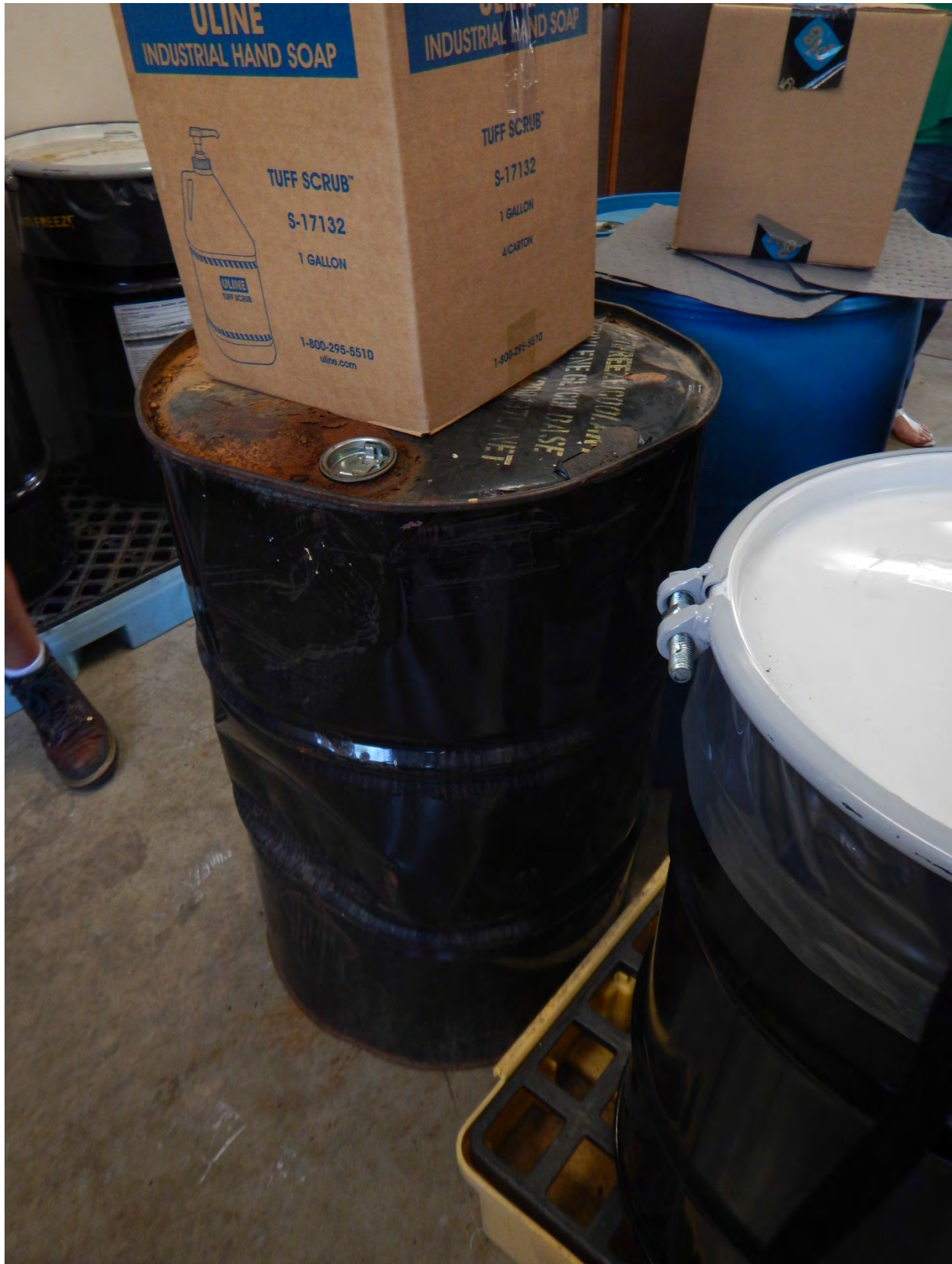
420 – Dented antifreeze drum with corrosion on top building 1570
