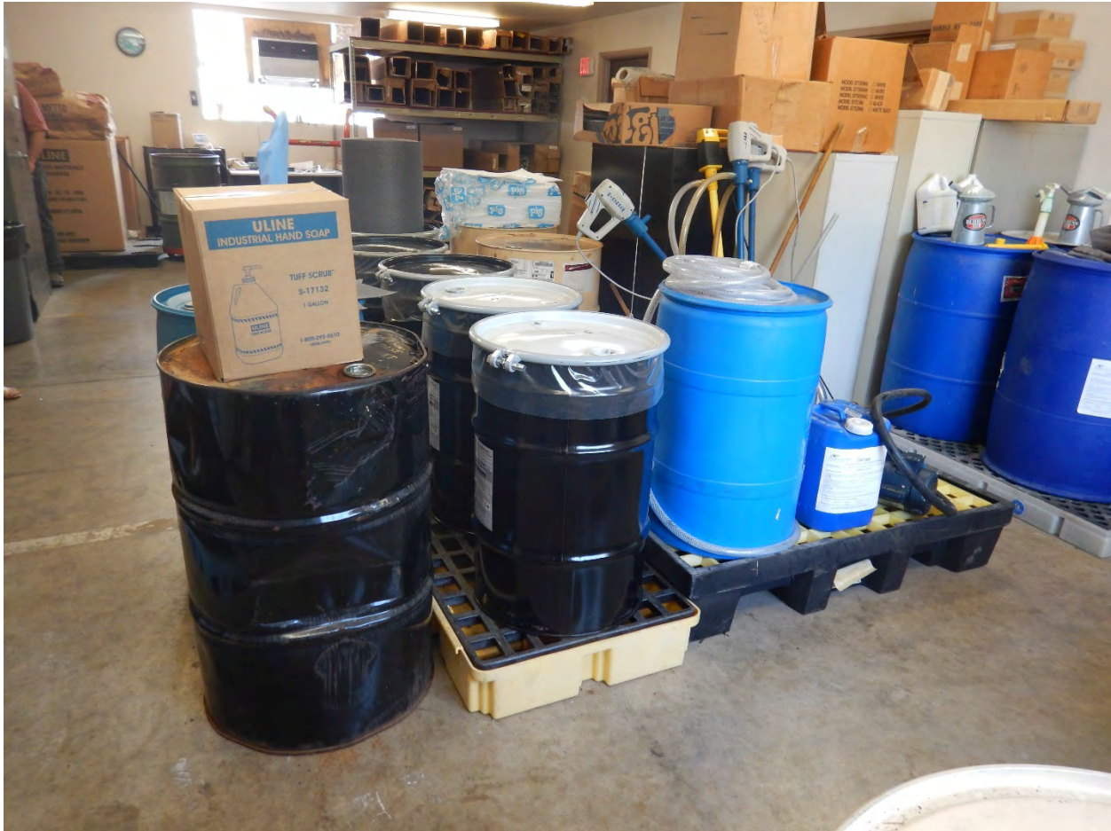
419 – Dented antifreeze drum with corrosion on the top building 1570
