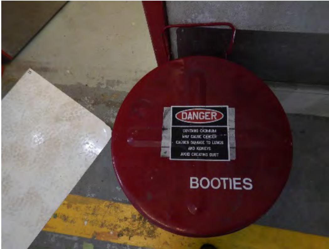
479 – PPE collection from blast area in building 282
