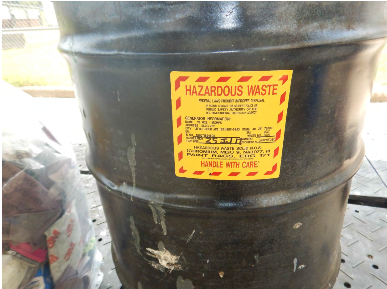
448- Hazardous waste in 90-day accumulation area outside building 282
