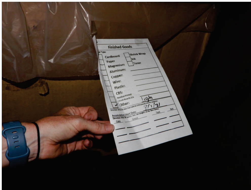
Photo 5 (DSCN0126.JPG): Label and accumulation start date on gaylord holding universal waste lamps seen in photo 6.
