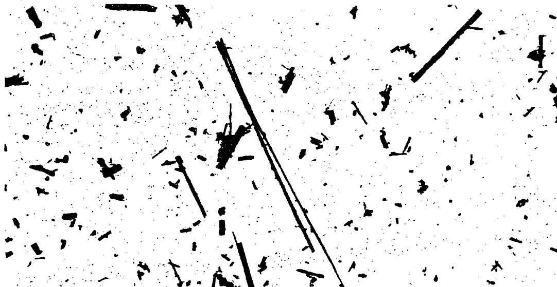
Electron micrograph of barroisite after grinding to produce fine dust (magnified approximately 4,500 X; 1 cm equals 2.2 \mu )
