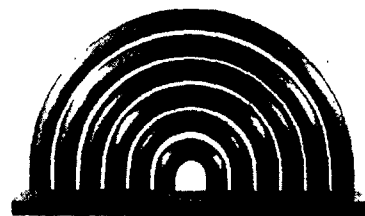
End Section of Heating Element U-Bend 1\frac{1}{4} " Copper Tubing 16-gauge showing full \frac{1}{2} " bridge between each tube and thru clearance for cleaning between rows.
