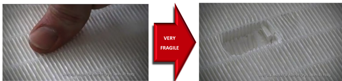
Figure 6.2: Glass fiber media can be easily damaged.
