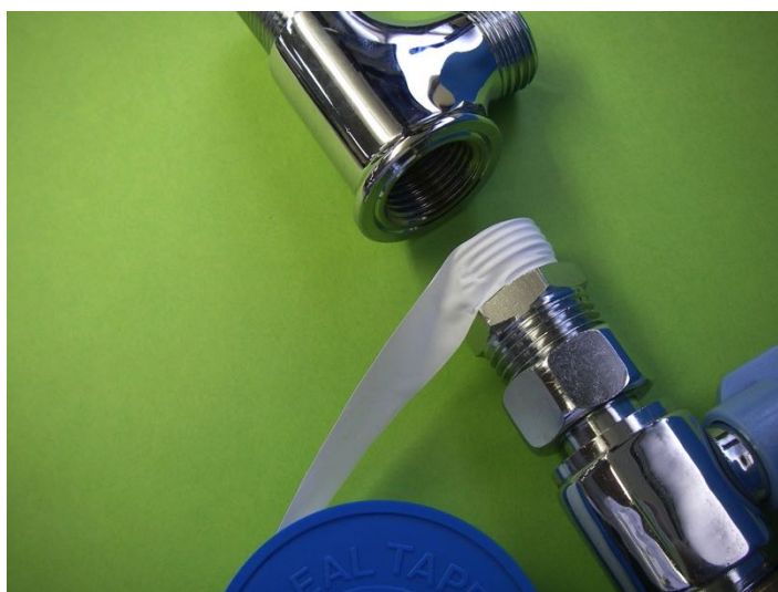
Figure 5.1: Sealing tape for fittings in the household.
