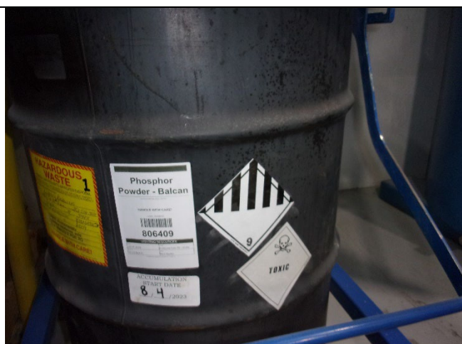
Figure 14: 12:47 PM Balcan Room One 55-gallon SAA container of phosphor powder observed with hazardous waste label and indication of the hazards of the contents.
