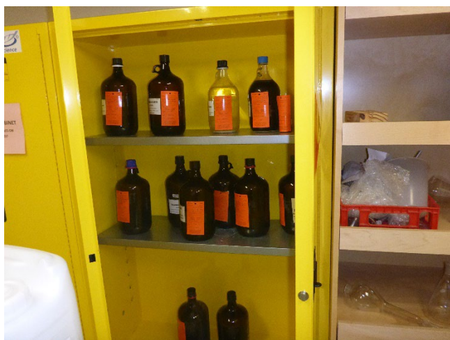
Photo 6: One of two flammable cabinets holding twelve 2-liter bottles of hazardous waste in the Solvent Room.
