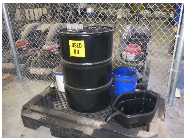
Photo 9: Secondary containment pallet holding one 55-gallon drum of used oil, which was labeled with the words "used oil," in the Landscaping / Grounds Maintenance Area.
