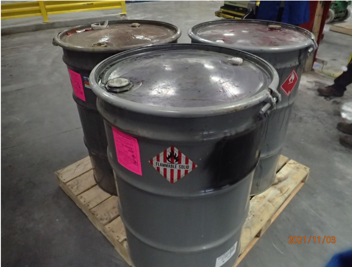
Photo 2: Three (3) 55-gallon drums of paint-contaminated debris generated from three different washes of machinery. The containers were closed, labeled, dated, and marked with an indication of hazard. The containers were on a pallet to be sent to the 90-day central accumulation area.
