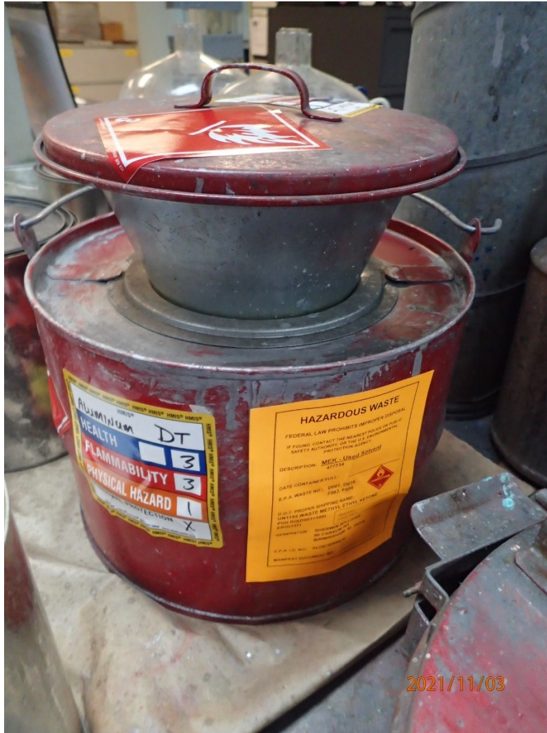
Photo 16: Two (2) 5-gallon containers of dirty thinner containing aluminum, closed, marked with an indication of hazard but missing a “Hazardous Waste” label. The hazardous waste labels were added to the two containers that were missing it during the inspection.
