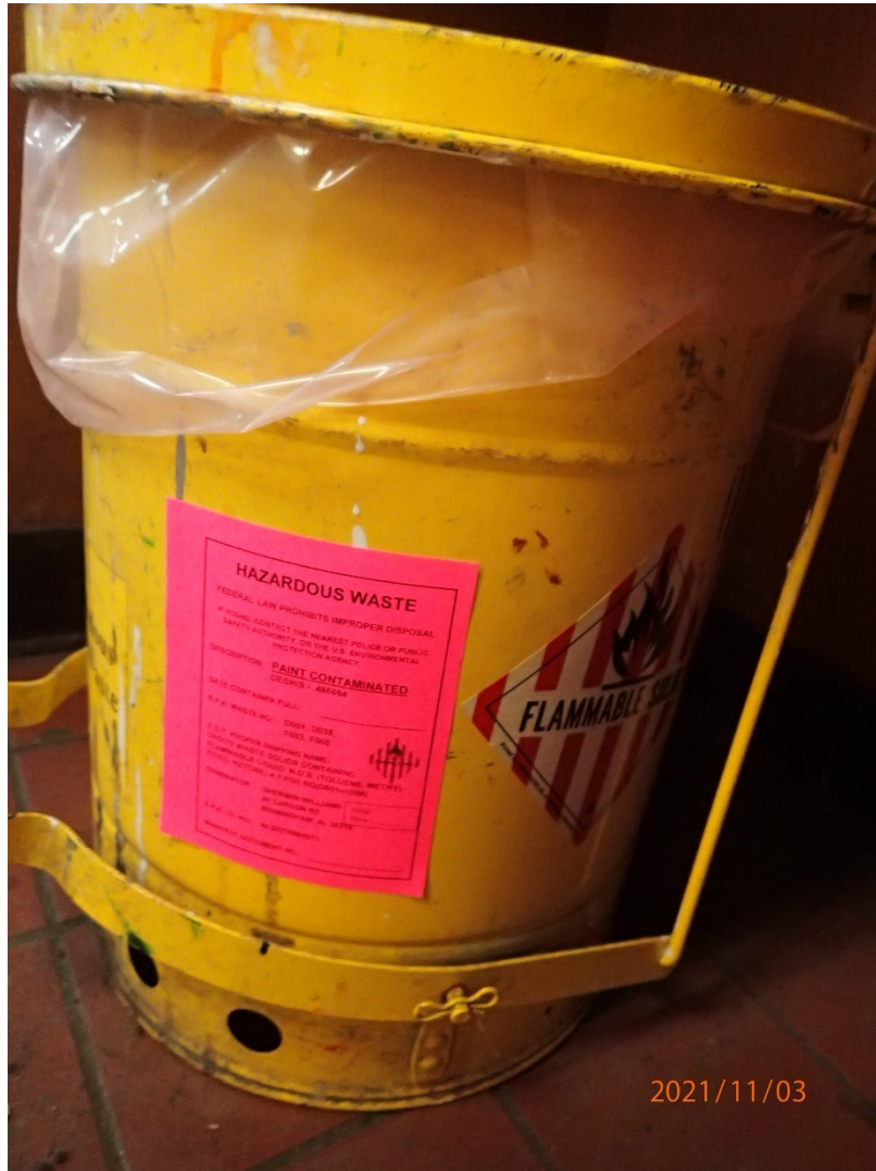
Photo 15: Six (6) 5-gallon containers of hazardous waste solids, closed, labeled “Hazardous Waste”, but missing a marking for an indication of hazard. New hazardous waste labels that included an indication of hazard were placed on the six containers missing an indication of hazard during the inspection.
