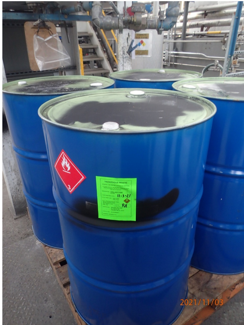
Photo 7: Four (4) 55-gallon drums of solvent still bottoms, closed, labeled "Hazardous Waste", marked with an indication of hazard, and dated 11/3/2021.
