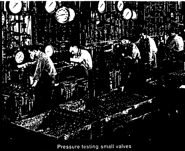
Pressure testing small valves
