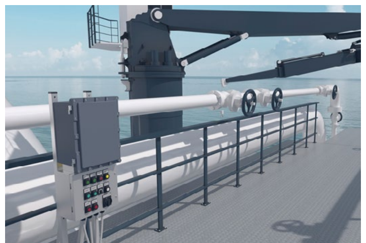
A flanged Ex de enclosure solution from Pepperl+Fuchs, in which electrical components can be safely operated in hazardous areas, is ideal for safe operation of the crane control system when loading and unloading the gas tanker.
