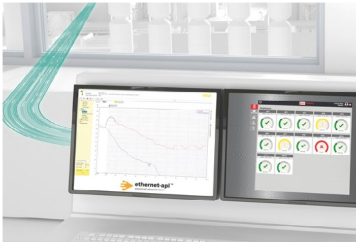
With Ethernet-APL, the data from the field devices is transmitted fast and digitally via the two-wire cable in real time, giving authorized users an overview of the system status at all times.
