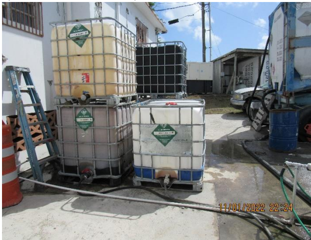
IMG 784 -Observed totes of chemical additives with connective application hoses by stormwater into the ready-mix concrete manufacturing process.
