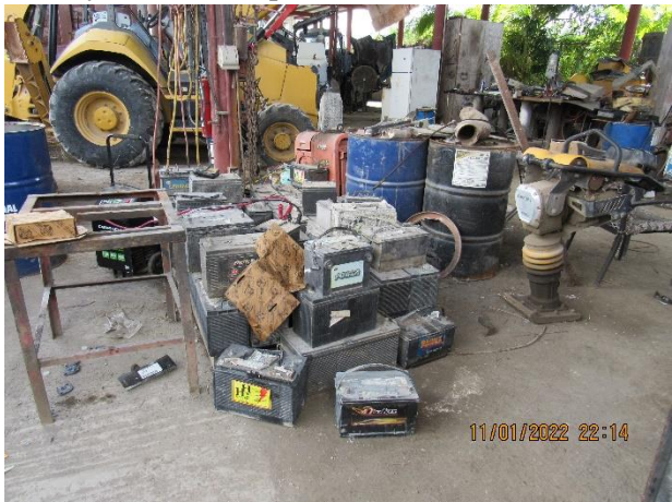
IMG 771 -Accumulation of spent auto batteries situated on floor of maintenance shed in potentially managed under incompatible conditions.
