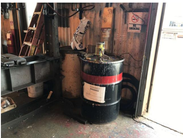
Photo 26: BD034 Maintenance aerosol can puncture device.
