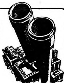
5 Two-stage unit has high-voltage wire for charging electrode; flat plate for precipitating; screen for collecting
