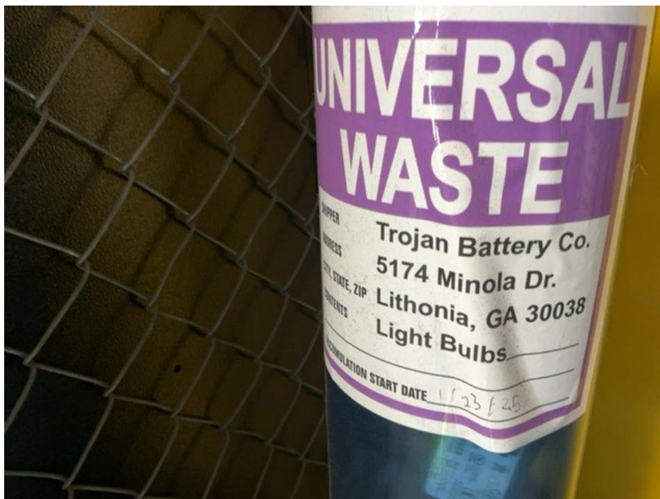
Photo 9 – Label on the universal waste battery containers incorrectly marked as universal waste lightbulbs observed during the CEI.
