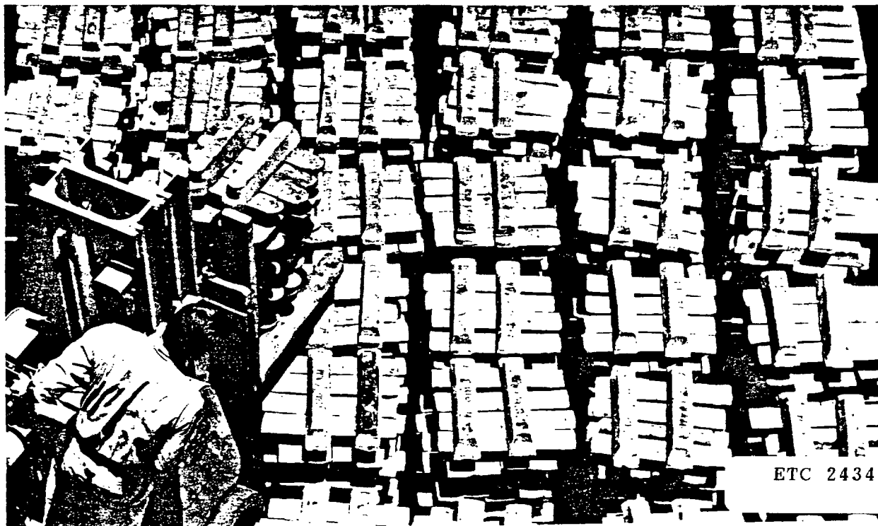
Lead bars at one of the Ethyl manufacturing plants. Pig lead is the prime raw material of tetraethyl lead
