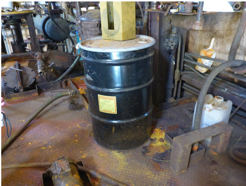
Photo 7: One 55-gallon drum in the Potassium Room platform SAA for managing hazardous waste filter cloths that are generated in the production process. The drum was closed and labeled D007 / D009 hazardous waste solids, but it was not marked with an indication of the hazards of its contents.
