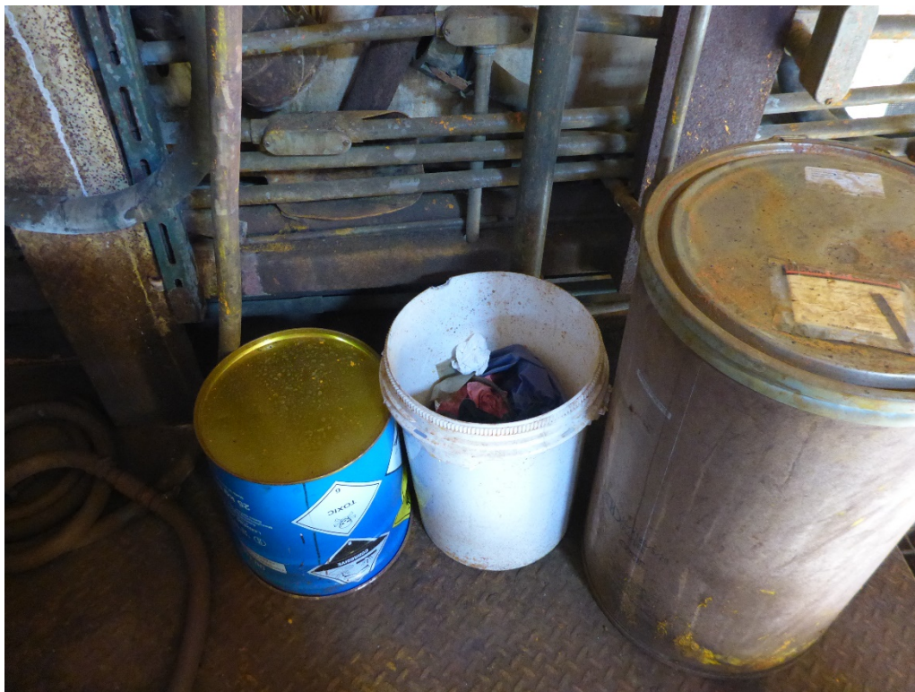
Photo 8: One 5-gallon bucket on the platform in the Potassium Room for accumulating hazardous waste used PPE, gloves and trash. The drum bucket was not closed or labeled, and this area was not identified as a SAA.
