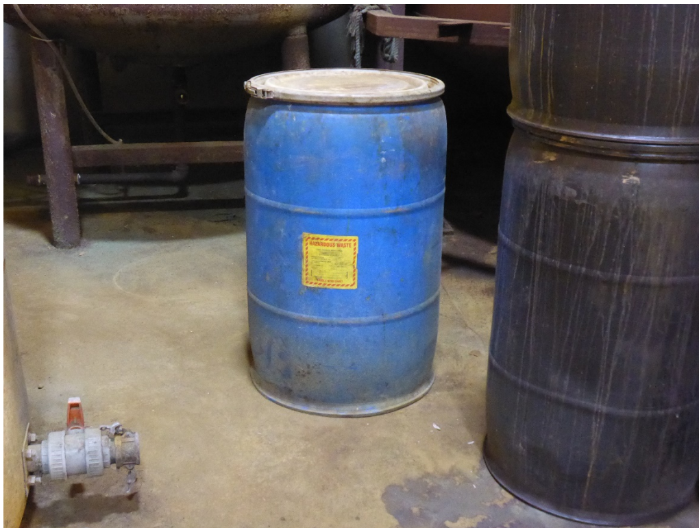
Photo 6: One 55-gallon drum on the floor in the Potassium Room SAA for managing hazardous waste used PPE, gloves and trash. The drum was closed and labeled D007 / D008 hazardous waste solids, but it was not marked with an indication of the hazards of its contents.
