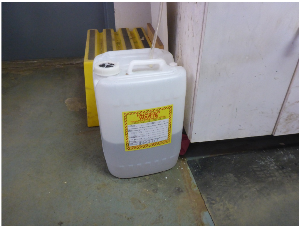
Photo 10: One 5-gallon carboy in the Laboratory SAA for managing hazardous waste lead chromate liquid that is generated by the Atomic Analyzer. The container was closed and labeled hazardous waste liquid, but it was not marked with an indication of the hazards of its contents.
