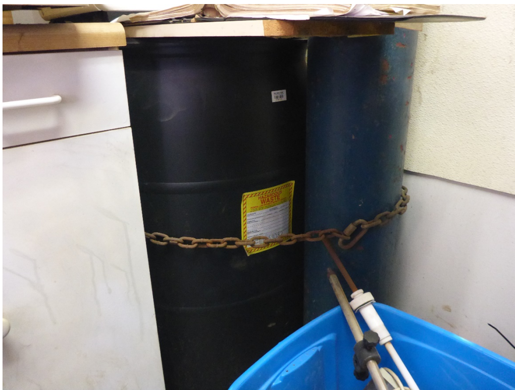
Photo 9: One 55-gallon drum in the Laboratory SAA for managing hazardous waste lead chromate liquid that is generated by the Atomic Analyzer. The drum was closed and labeled hazardous waste liquid, but it was not marked with an indication of the hazards of its contents.
