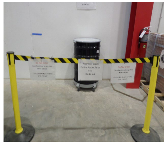
Corning. Waste Salt CAA. The inspectors observed one 55-gallon container storing hazardous waste potassium nitrate (D001) in the CAA at the time of the inspection. Photograph 12 taken at 2:34 p.m.
