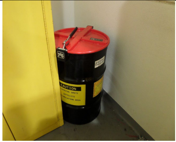
Corning. Mold Shop. The inspectors observed one 35-gallon container storing aerosol cans labeled as hazardous waste. The inspectors observed the container was not marked or labeled with an indication of the hazards. Photograph 10 taken at 12:33 p.m.
