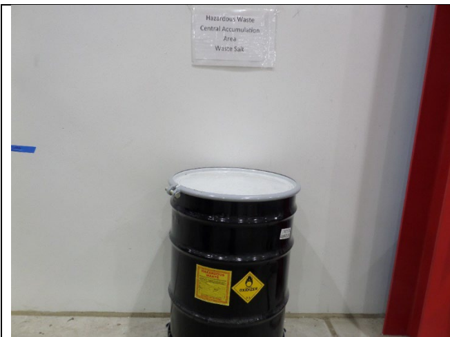
Corning. Waste Salt CAA. The inspectors observed one 55-gallon container storing hazardous waste potassium nitrate (D001) in the CAA at the time of the inspection. Photograph 11 taken at 2:34 p.m.
