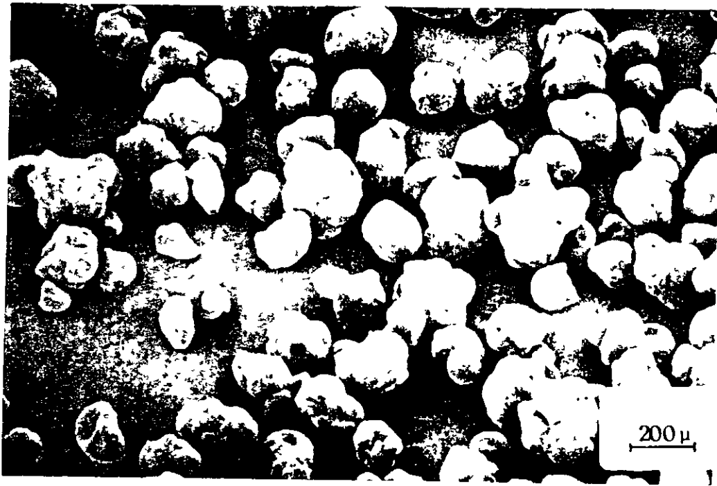
Figure 5. Suspension PVC grains: 50X.
