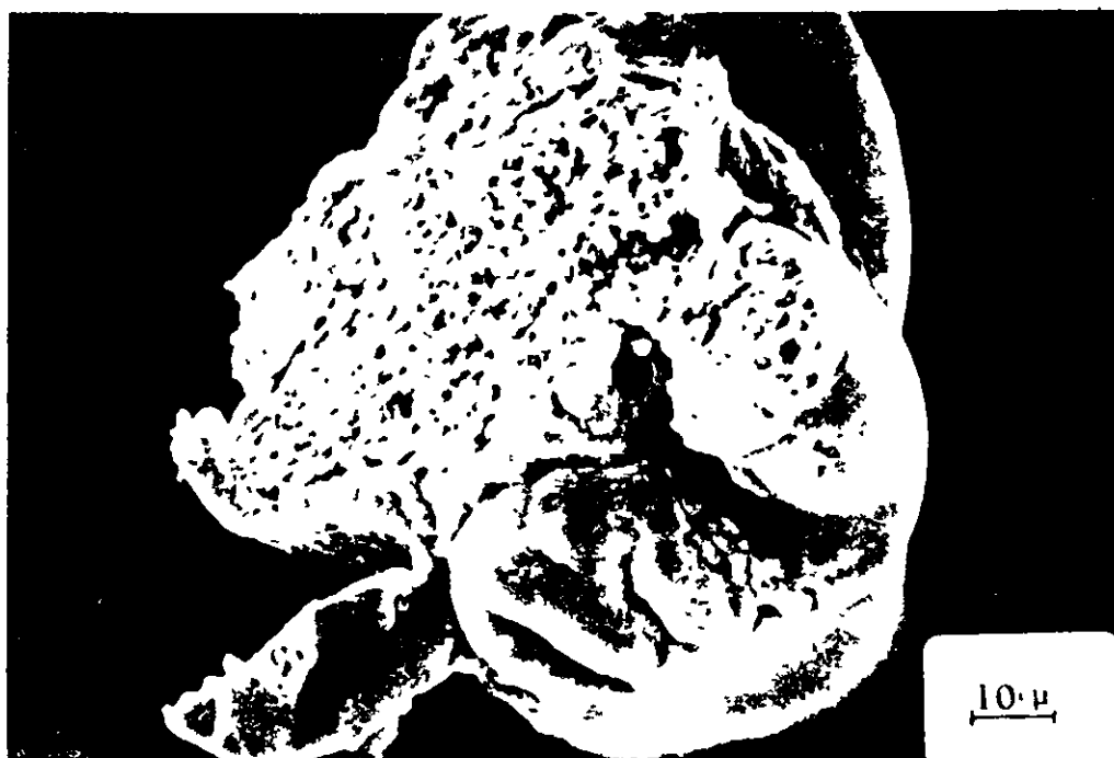
Figure 8. Interior structure of a suspension PVC grain: 800X
