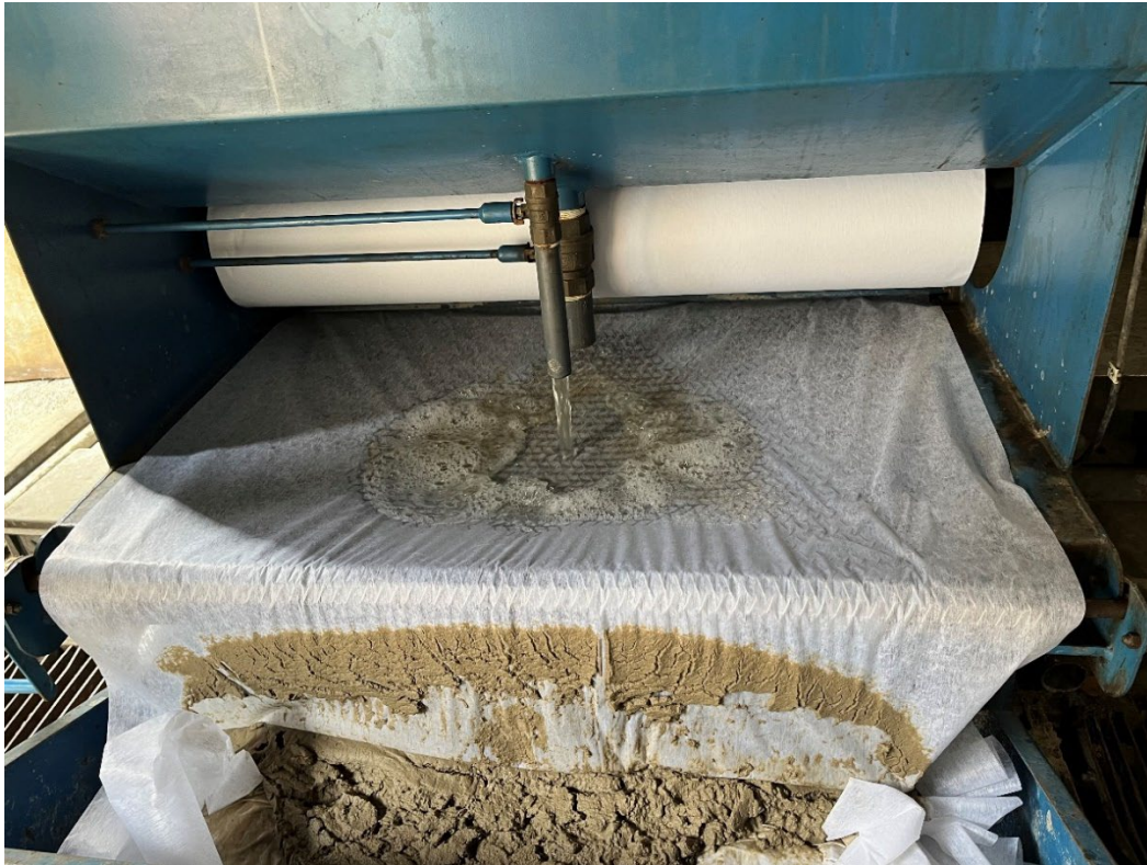
Photo #8. Effluent from the reactor chamber discharges onto the cloth paper filter.
