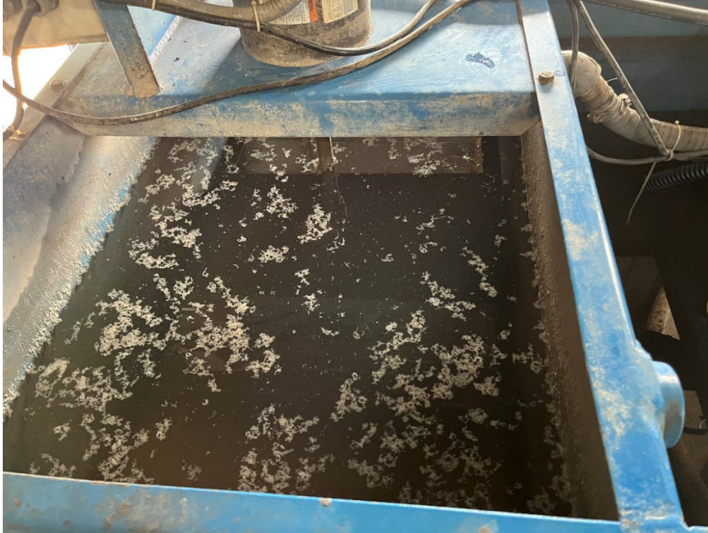
Photo #7. Polymer is added into the reactor chamber while the agitator provides mixing.
