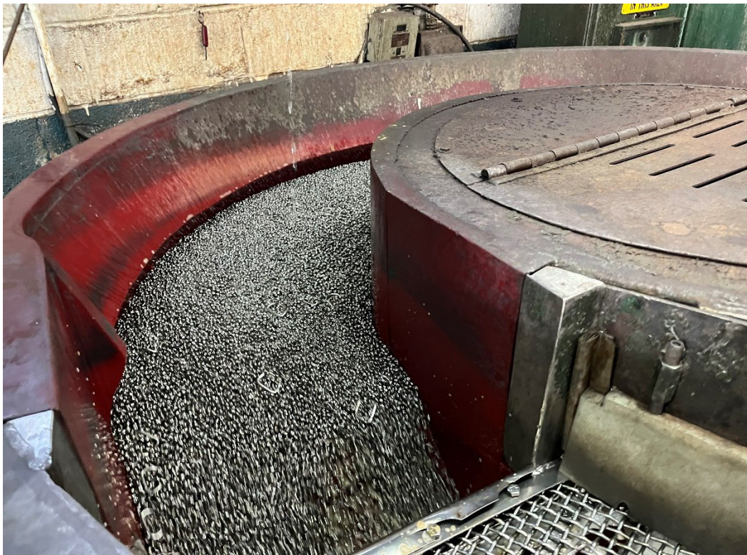
Photo #1. Municipal water is used in the tumbler to clean and polish bare metal parts.
