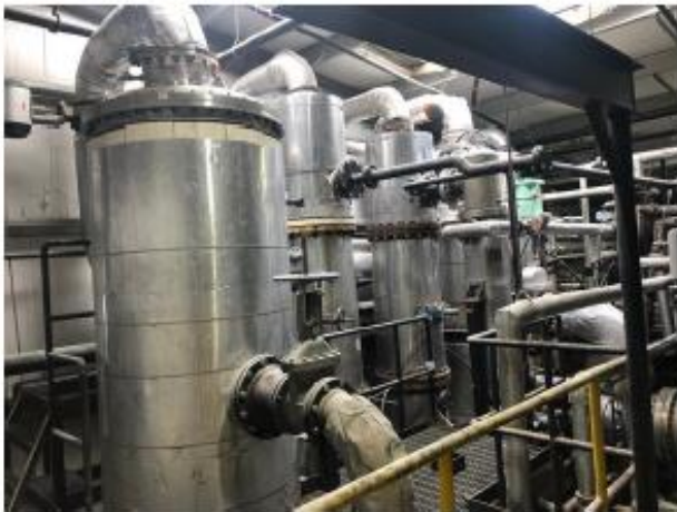
Production Flash Dryers. From left to right: Acid Esterification Dryer; Feedstock Dryer; Biodiesel Dryer; Glycerin Dryer #1, and; Glycerin Dryer #2.
