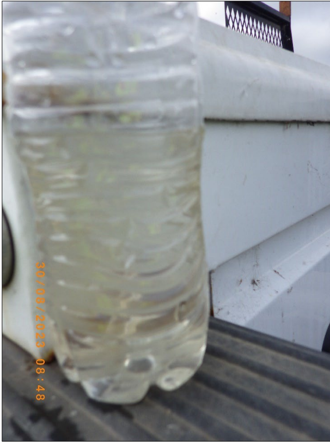
Photograph 123. DTE - Monroe Plant RIMG3200.JPG Description: View of water collected by a facility representative using a plastic bottle for a visual aid regarding the darker colored water in discharge canal by 001H. Note this is not the bottle or sampling method that would be used for NPDES compliance samples.
