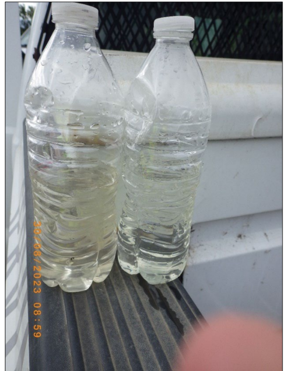
Photograph 126. DTE - Monroe Plant RIMG3203.JPG Description: View of water collected from the dark colored water in the discharge canal by 001H on the left and downstream by 001 on the right. The water was collected by a facility representative for a visual aid during the inspection, these are not the bottles or sampling method that would be used for NPDES compliance samples.
