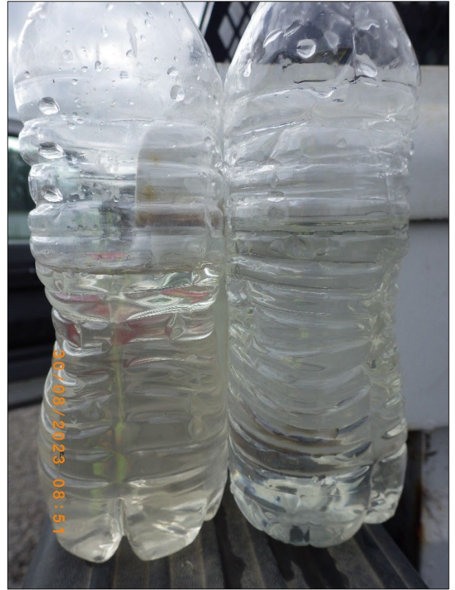
Photograph 124. DTE - Monroe Plant RIMG3201.JPG Description: View of water collected from the dark colored water in the discharge canal by 001H on the left and downstream by 001 on the right. The water was collected by a facility representative for a visual aid during the inspection, these are not the bottles or sampling method that would be used for NPDES compliance samples.
