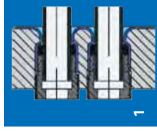
Fig. 3: Double tubesheet shellside and tubeside glass-lining
