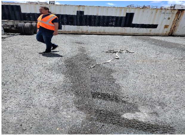
IMG 6966 -Flow path of stormwater flow in the rear yard area of the maintenance shed.
