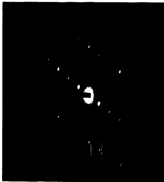
Figure 1b. SAED pattern of a talc ribbon with its (001) face oriented approximately parallel with the electron beam.
