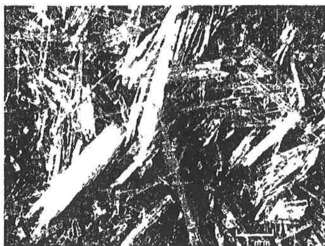
FIGURE 23. - Macrophotograph of tremolite showing prismatic and acicular crystal shapes (X 10).
