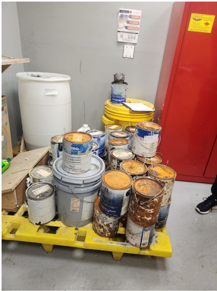
Photo #1 – waste paint cans and unlabeled 30-gallon container of paint thinner consolidated in Building 4. Inspectors observed one acrylic waste paint can was not marked with a hazardous waste label.
