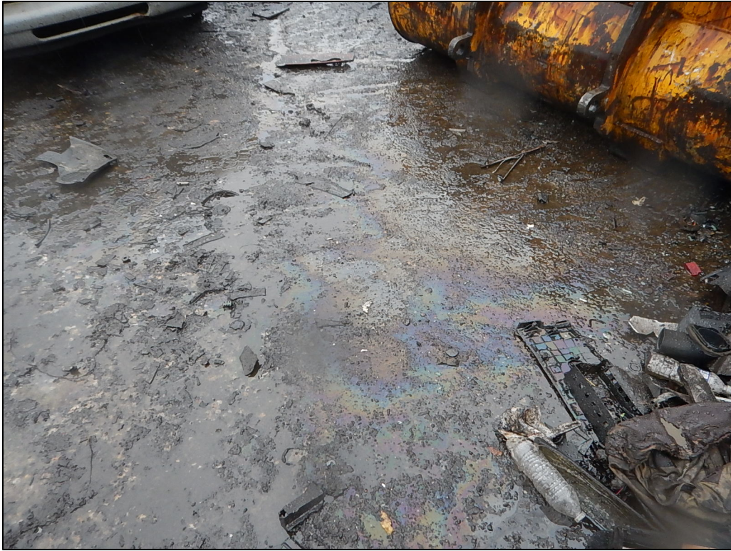
DSCN3882. View of petroleum sheen adjacent to the crusher. Runoff from this area was flowing toward the southwest perimeter.
