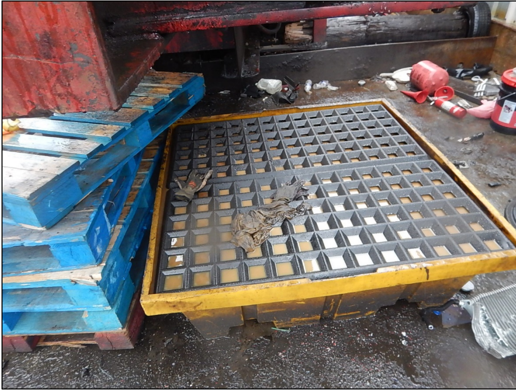
DSCN3878. View of a containment pallet located next to the crusher. The pallet was full of rainwater and not being used to contain anything.
