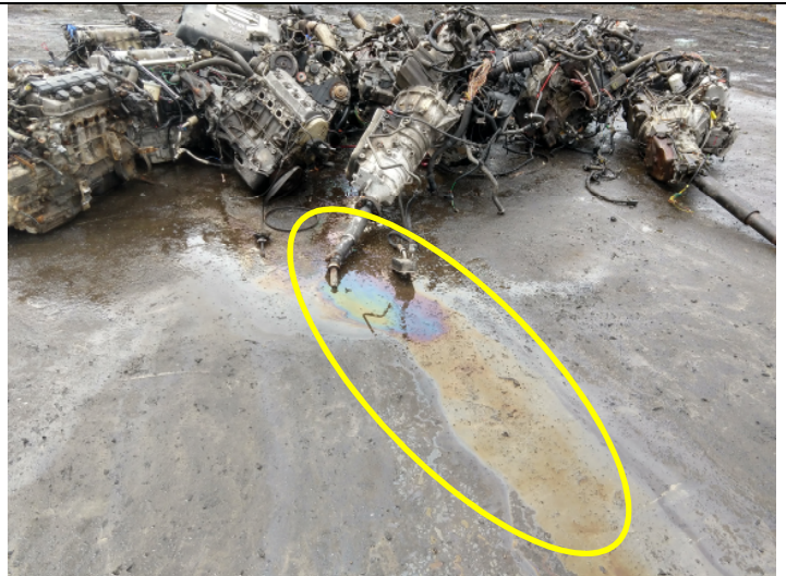
8) Oil Sheen at the Crusher
