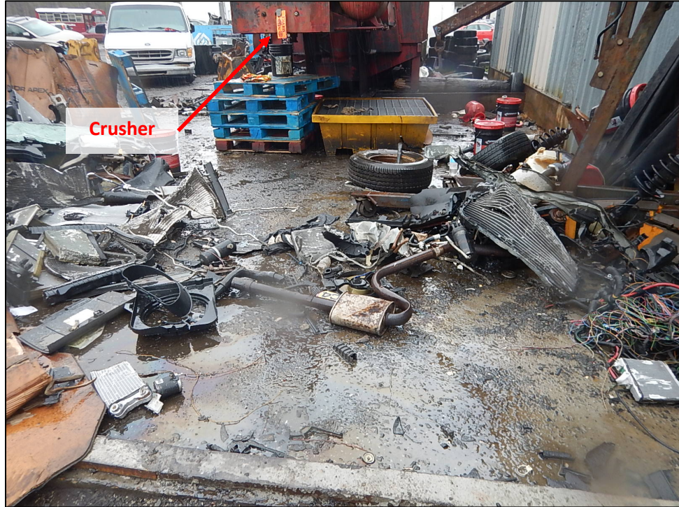
DSCN3876. View of the crusher in the southeastern area of the Facility and the car waste. The crusher was located on a concrete pad but was uncontained. Petroleum staining and residue was observed covering most of the pad.
