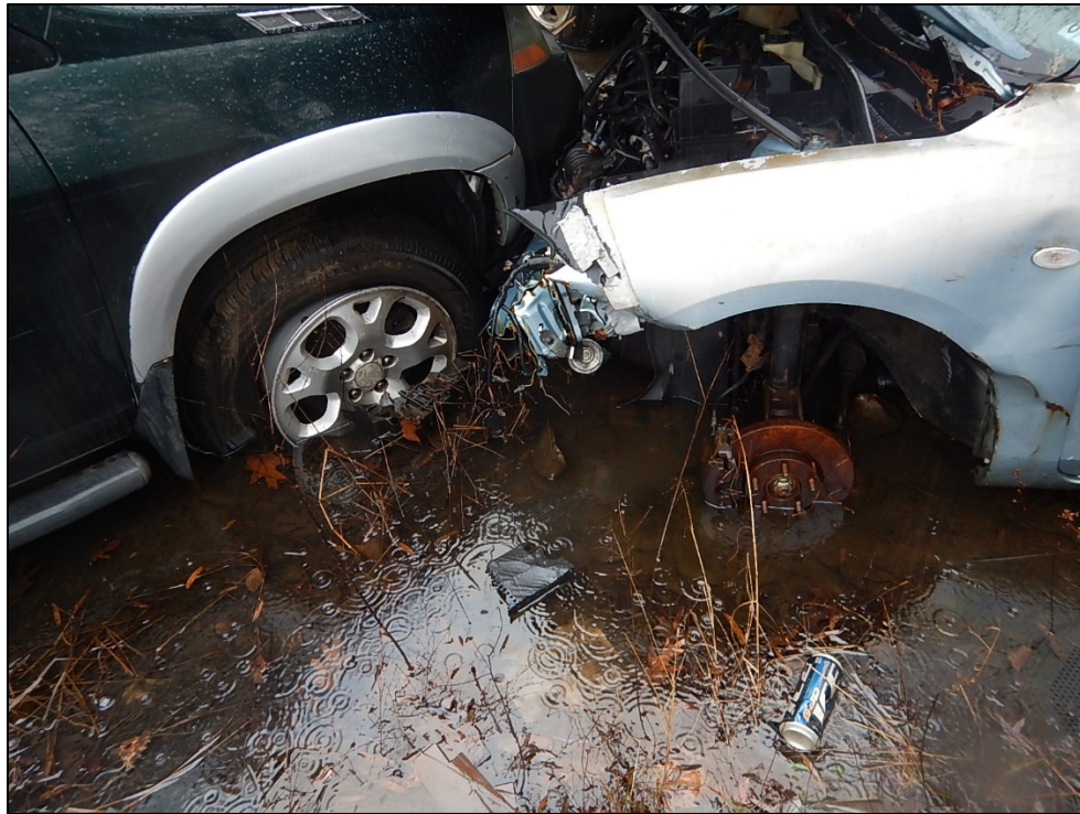
DSCN3840. View of the two vehicles in the southwestern part of the lot with stormwater pooled underneath them, around rusted wheel/brake components.
