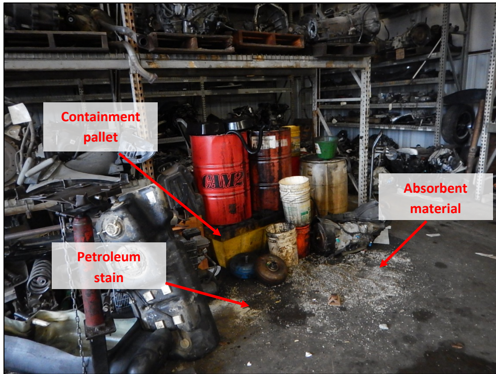
DSCN3717. View inside the dismantling garage of drums used to collect drained fluids. Note that fluids had leaked outside the containment pallet.
