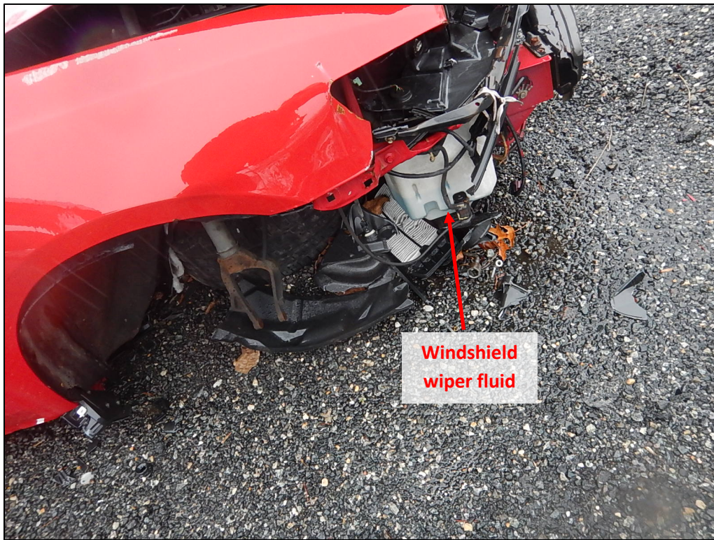
DSCN3835. View of a vehicle stored in the southwestern part of the lot with windshield wiper fluid remaining in the reservoir.
