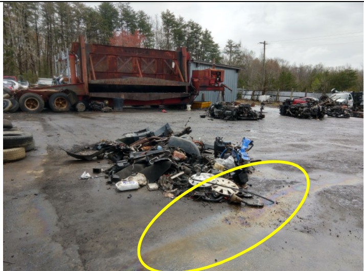
7) Oil Sheen at the Crusher
