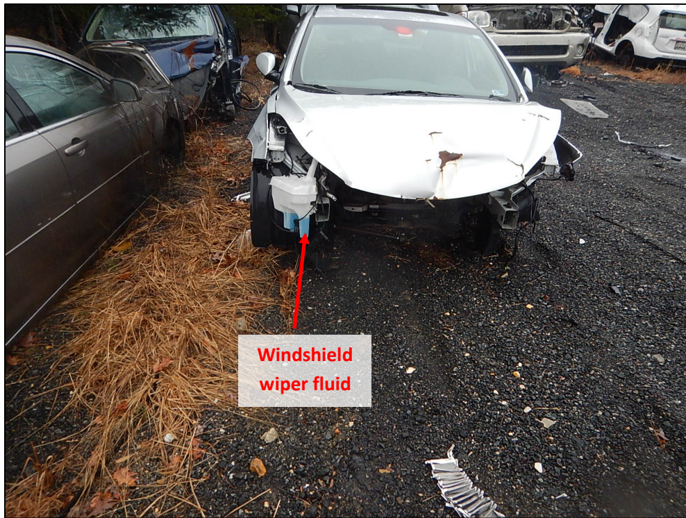
DSCN3832. View of a vehicle stored in the southwestern part of the lot with windshield wiper fluid remaining in the reservoir.
