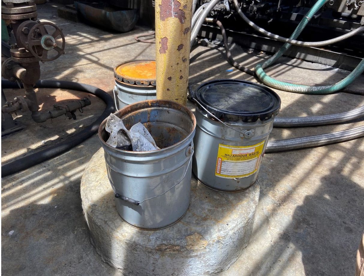
Figure 1: Three 5-gallon satellite hazardous waste drums were not properly labeled in the Column Pad. Two of the drums were also not properly closed.
