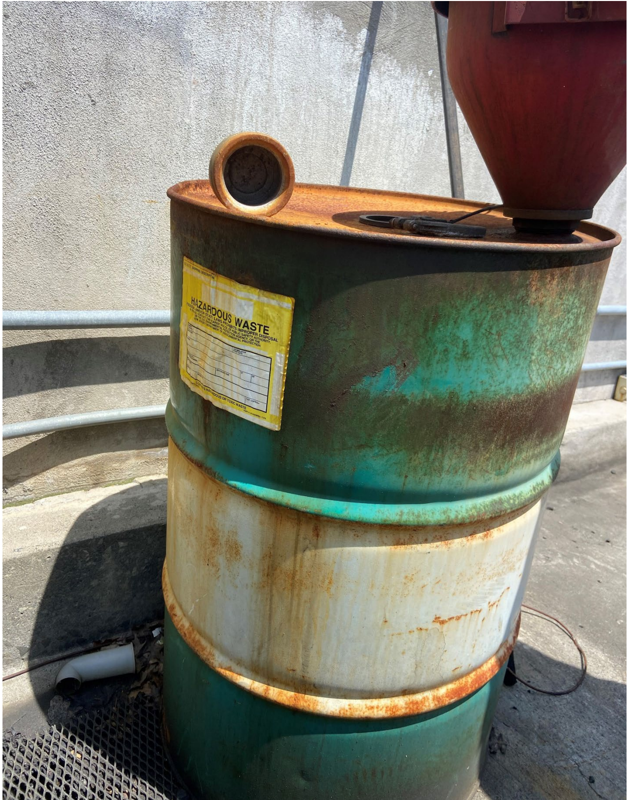
Figure 5: Corrosion and improper labeling on 55-gallon hazardous waste drum outside the Column Pad.
