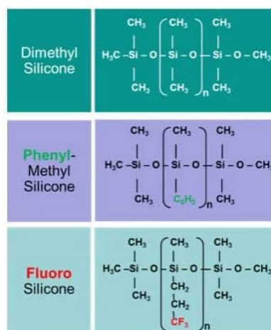
Figure 2: Dimethyl silicone (top). Phenyl-methyl silicone (middle). And Fluorosilicone (bottom)
