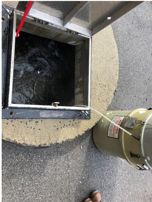
Photo #2. The RO retentate was sampled from the Ellicott Street Discharge monitoring location (Outfall 002).
