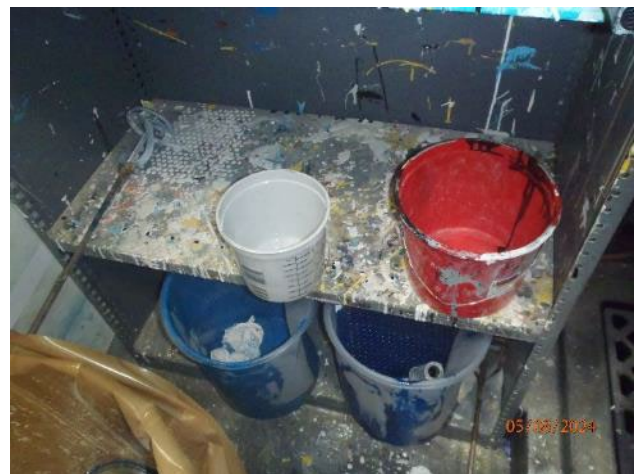
Picture 10 – Painter Cleanup SAA epoxy paint allowed to dry
