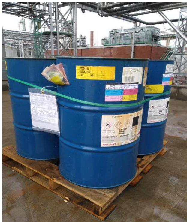
Photo 4: Building 244 Courtyard: Four drums of hazardous waste were not labeled “Hazardous Waste” at the time of the inspection.
