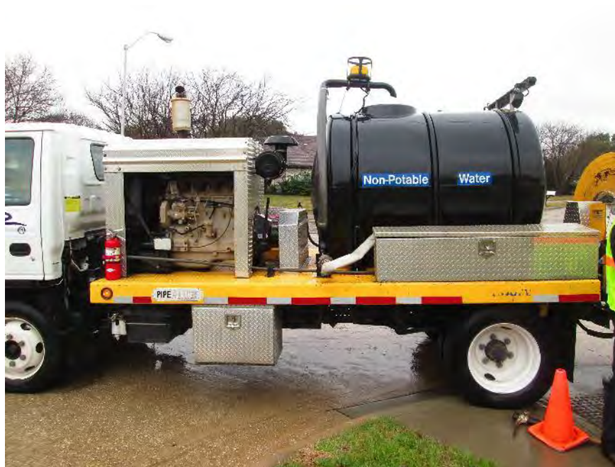
Photograph 32. Jet Truck Crew – View of one of the City's three jet trucks.
