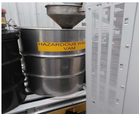
Photo-1 SAA Container (Missing Indication of Hazard Label (IOH))
