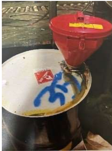
Photo #7 – Division 3 SA3-006, closed container (new funnel)
