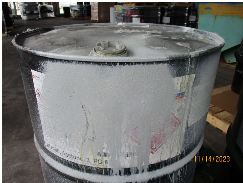
Photo #11 – Area of concern, label covered with paint
