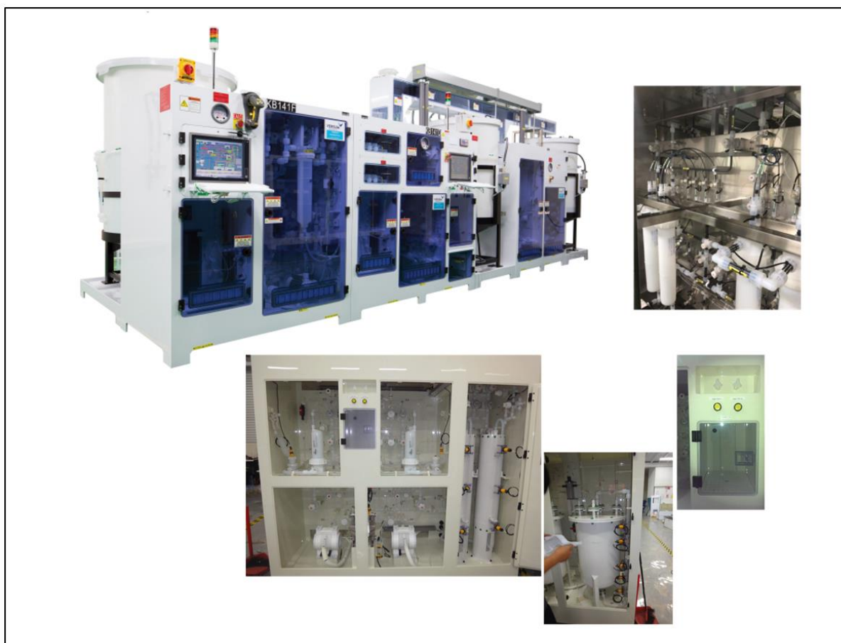
Figure 2: Example Pictures of different FlowMaster® Chemical Delivery Systems. Supplies precise blending and delivery of chemicals.
