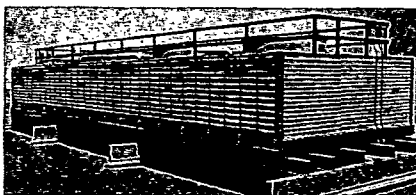
TYPE-20 CROSSFLO COOLING TOWERS: Induced draft, horizontal air flow units designed to meet low profile architectural requirements. Maximum height to top of fan stack is 8 feet. Capacity per cells range from 60 to 300 tons of refrigeration.
