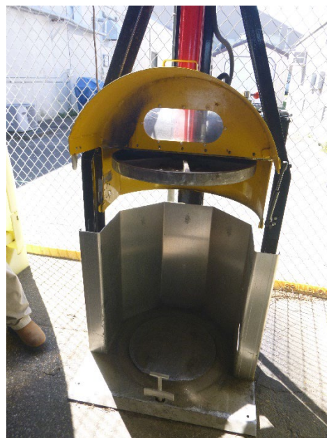
Photograph 31: HazMart CAA Compactor.
