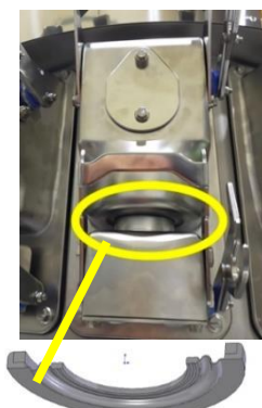
diaphragm example (sensor section)
