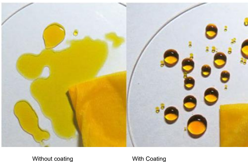
Figure 38 Difference among lens with coating and without coating 20
