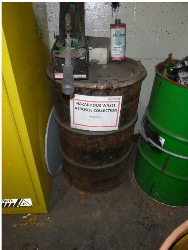
Photograph 1: Aerosol SAA Container with puncture device.
