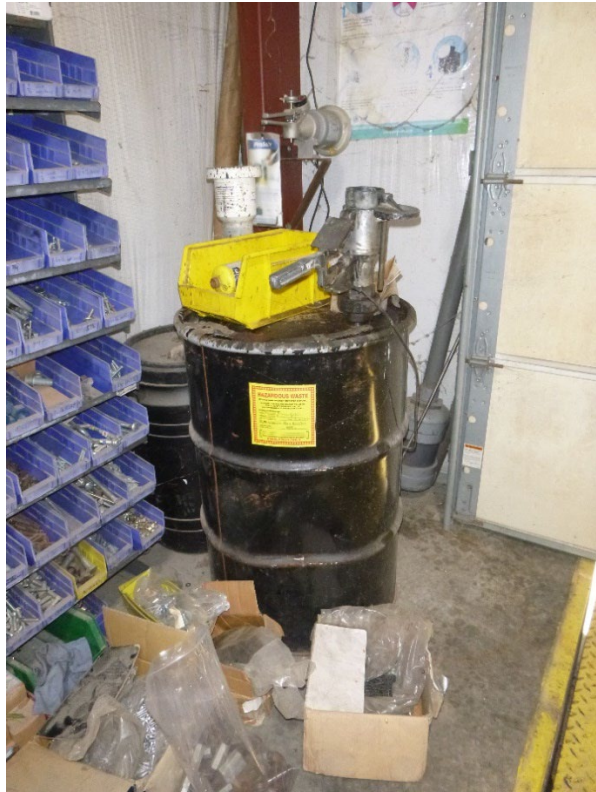
Photograph 2: Aerosol SAA Container with puncture device.
