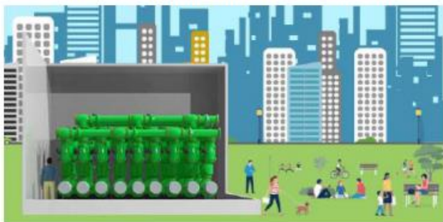
Figure 2 - Size comparison of typical substation for the 420 kV backbone of the European power grid, scaling consistent with Hitachi Energy product (left side) and a 420 kV air & vacuum circuit breaker concept presented in 36
