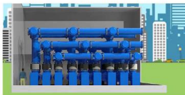
Figure 2 - Size comparison of typical substation for the 420 kV backbone of the European power grid, scaling consistent with Hitachi Energy product (left side) and a 420 kV air & vacuum circuit breaker concept presented in 36
