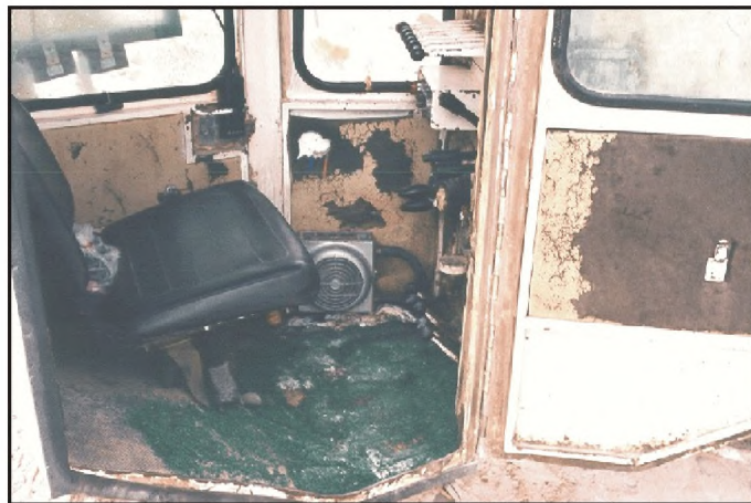
Figure 1.—Sweeping compound applied on drill cab floor with floor heater.
