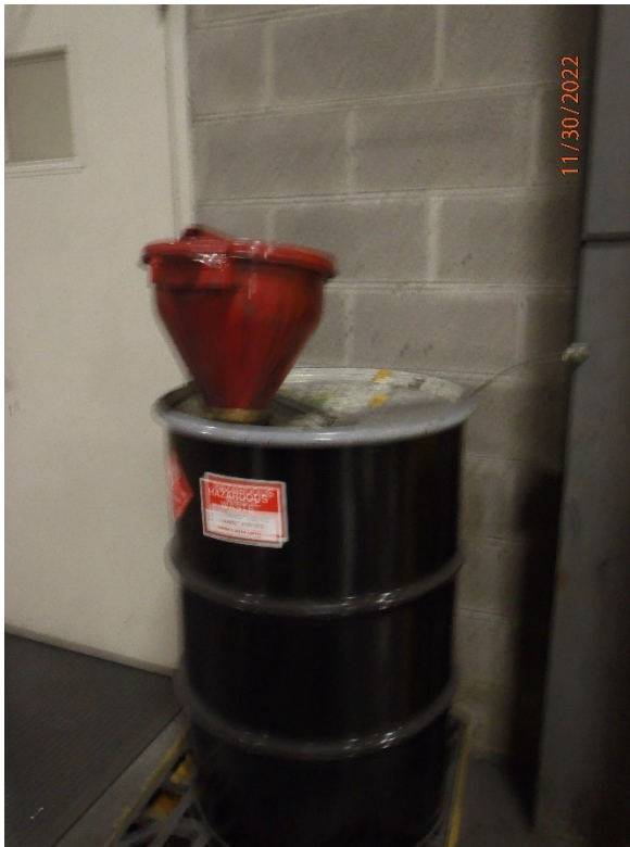
Figure 12: PB300021.JPG – Hazardous Waste SAA 55-Gallon Container
