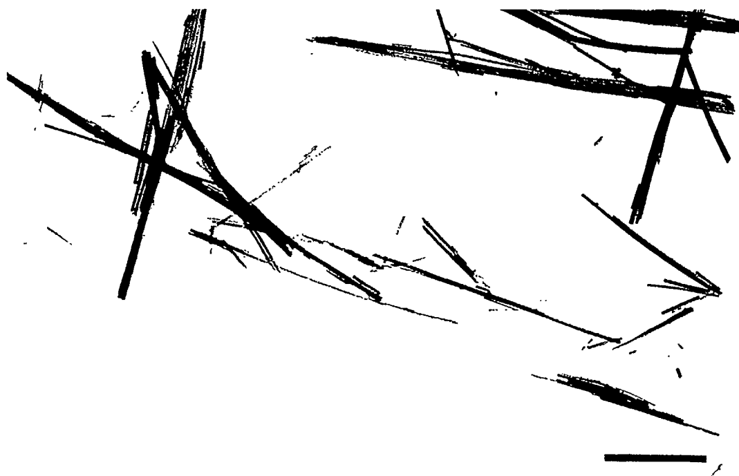
Fig. 2. Intrapulmonary chrysotile fibers in an ashed 25 \mu m thick section. Transmission electron microscopy. One day after administration. Scale = 1 \mu m.
