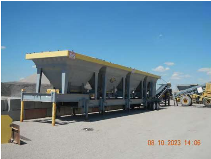
Photo #:01 (DSCN3385) Description: Photo of the aggregate storage bins associated with hot mix asphalt plant, currently staged and not operating.
