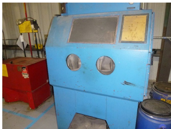
Photograph 4: Abrasive blasting unit and parts washer in the Maintenance Shop.
