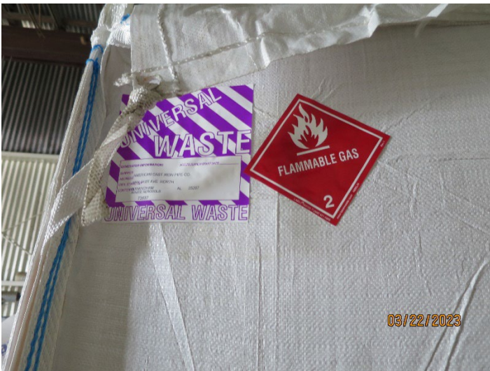
Photo 8: A cubic yard box of universal waste aerosol cans not marked with an accumulation date in the CAA.
