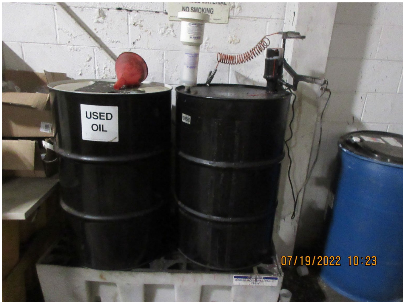
Photo 4 – SAA Area for Aerosol Cans and Used Oil collection container
