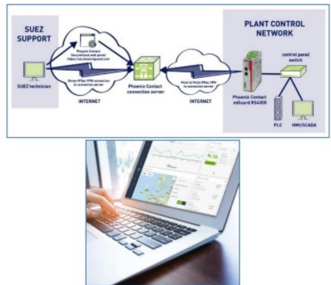
Figure 8: InSight* Remote Monitoring and Diagnostics with Cloud Based Analytics Package. Results available 24/7/365.
