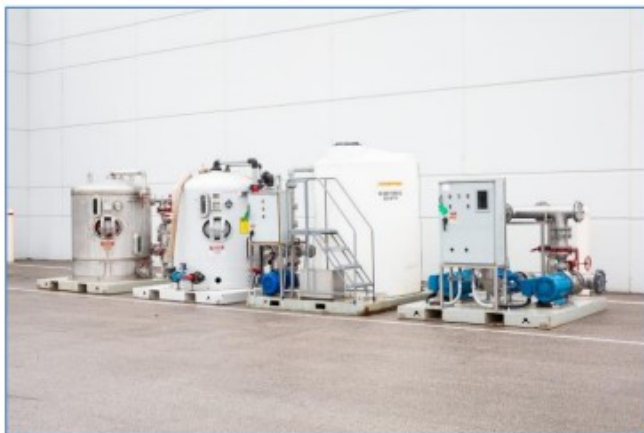
Figure 6: SUEZ proprietary multi vessel water purification system with interstage testing and automation control
