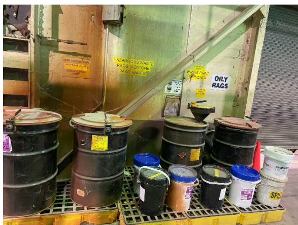
Photo-1 SAA and Universal Waste (Maintenance Shop)
